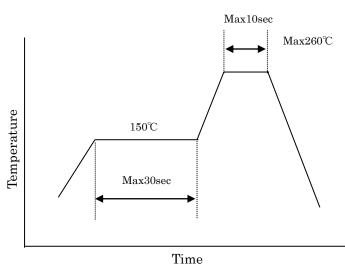
※Flow is within the limits only part of lead.※Flow of 2 times are possibleon condition that left temperature profile.
