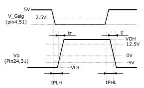
\*RG= $1.5\Omega$ , C\_load:0.33uF, f=10kHz, ON Duty=50%
