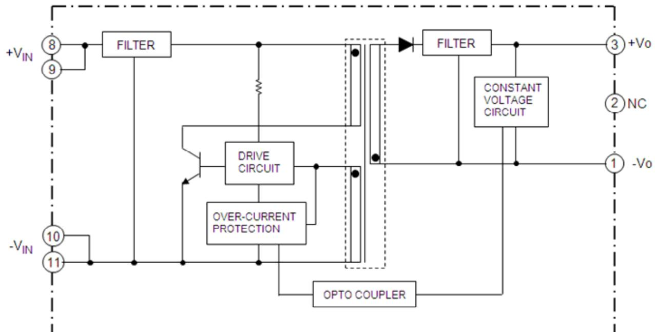
**ISOLATED TYPE DC-DC CONVERTER**
