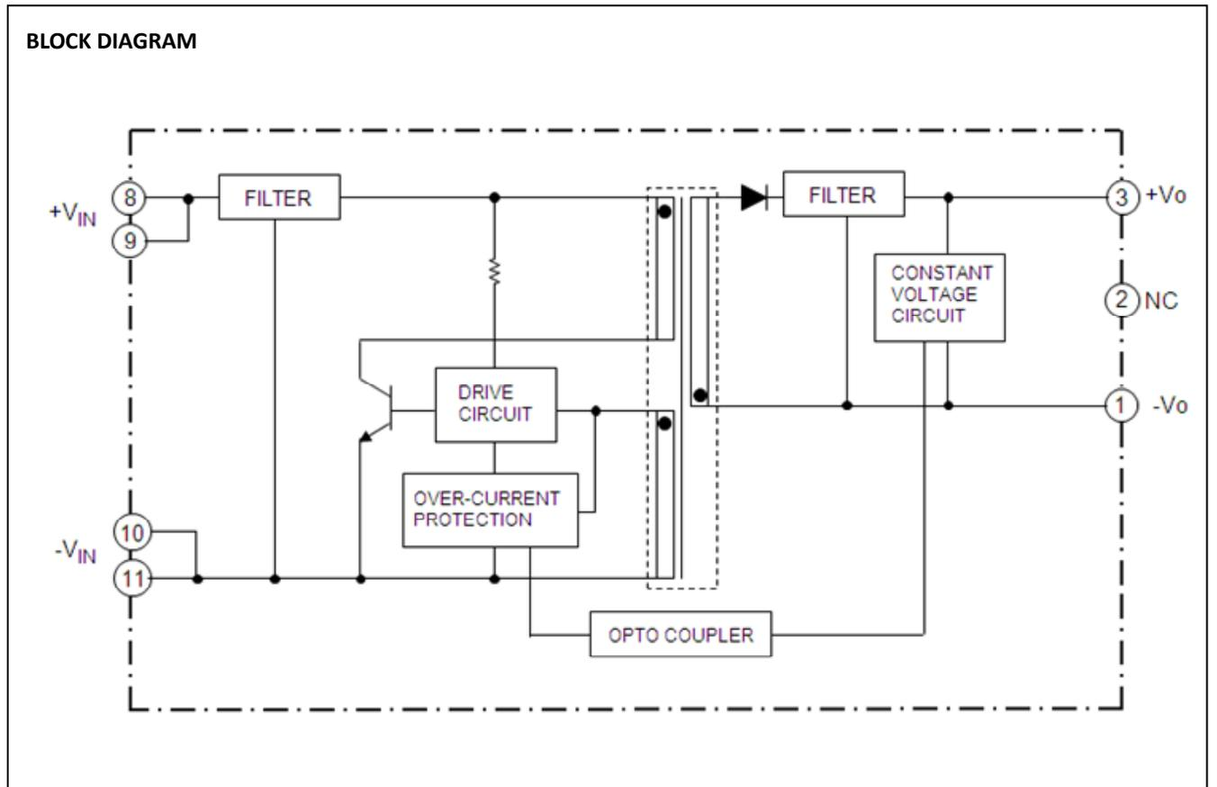
**ISOLATED TYPE DC-DC CONVERTER**
