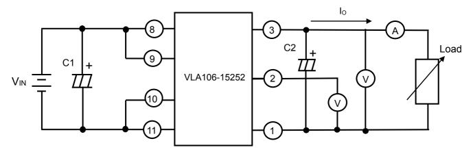
C1 :  $100\mu F$  50V (low impedance) C2 :  $47\mu F$  50V (low impedance)
