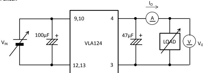
XIt is used the electrolytic capacitors which has the low impedance for output capacitor.
