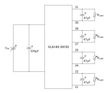
$\ensuremath{\mathbb{X}}$  It is used the electrolytic capacitors which has the low impedance fore output capacitor.
