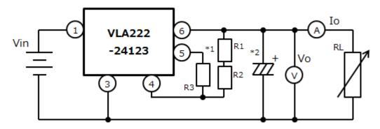
\*1 R1, R2 (tolerance 1%), R3(tolerance 5%),
