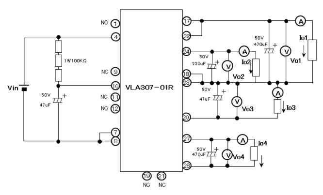
It is used the electrolytic capacitors which has the low impedance for output capacitor.
