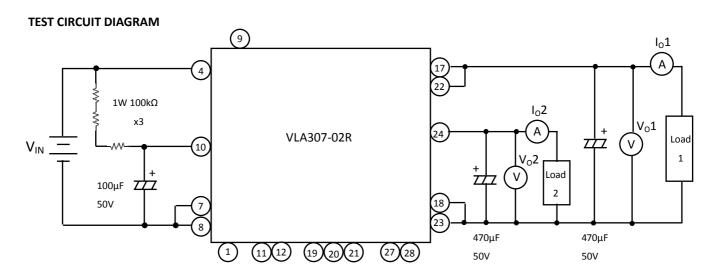
It is used the electrolytic capacitors which has the low impedance for output capacitor.
