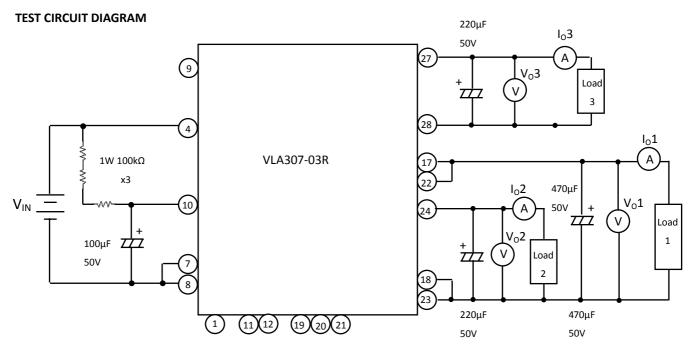
It is used the electrolytic capacitors which has the low impedance for output capacitor.
