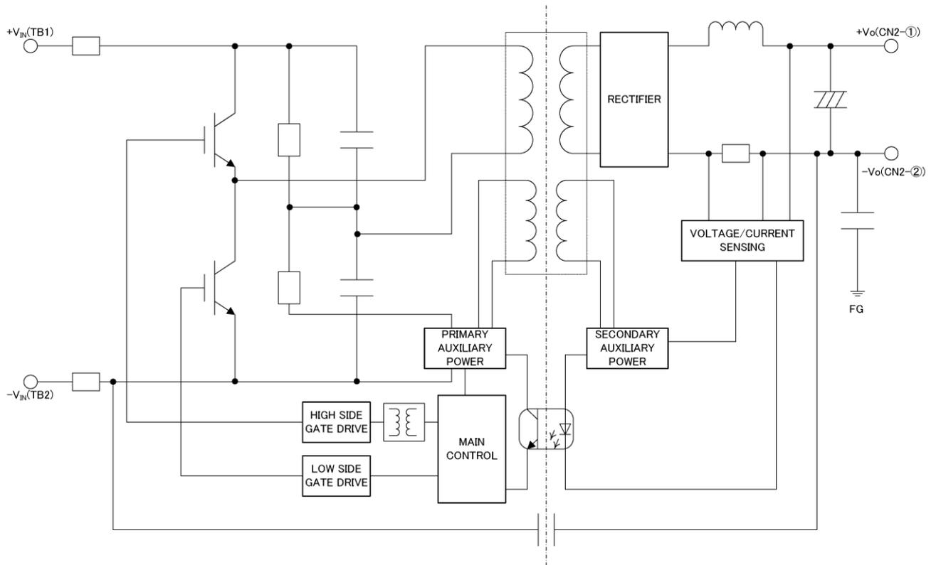
**ISOLATED TYPE DC-DC CONVERTER**
