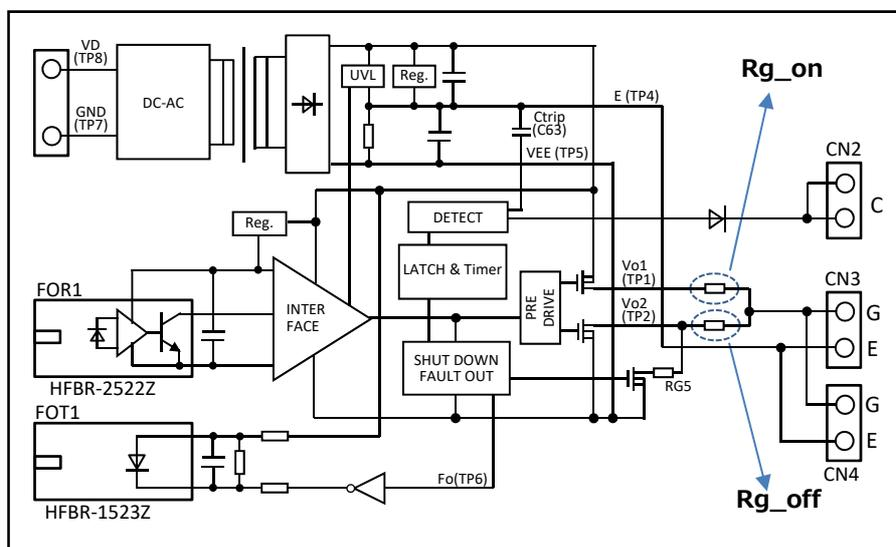
**ABOUT DISCHARGE RESISTOR FOR SOFT SHUT DOWN-ON ACTIVITY OF SHORT CIRCUIT PROTECTION**
