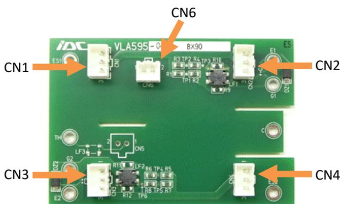
Pin No. assignment of connector
