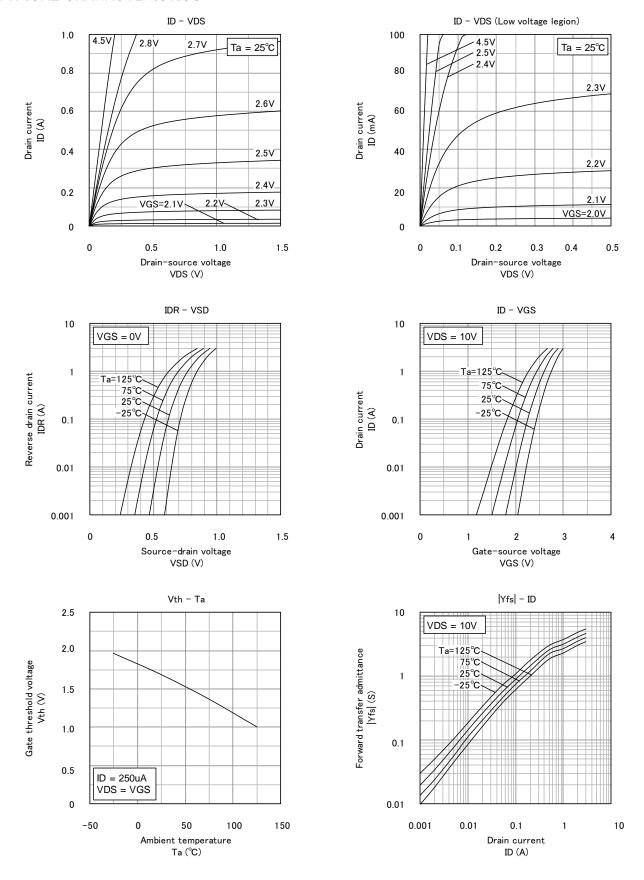
High Speed Switching Silicon N-channel MOSFET
