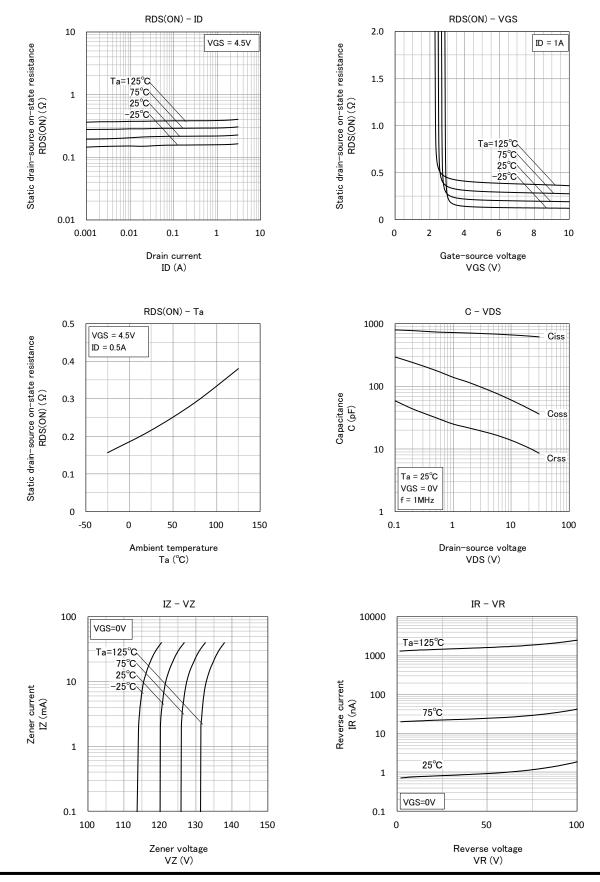
High Speed Switching Silicon N-channel MOSFET
