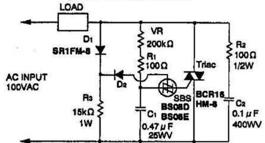
The above circuit is a triac phase control circuit making use of an SBS. In this circuit, an SBS gate is used to reduce the hysteresis characteristics. Thus, by using the variable resistance, phase control is possible over the wide range of 10 to 180 °C. Therefore, this circuit is widely usable in such applications as lighting control circuits, electric heater control, and other load control applications.
