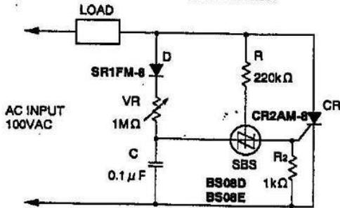
The above circuit is a thyristor phase control circuit making use of an SBS. In this circuit, using the SBS gate, the residual charge on C is reset, reducing the hysteresis characteristics. Therefore, over the range of the variable resistor, phase control (in the range 5 to 175°C) is possible, making this circuit widely useful in DC motor control and other control applications.
