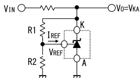
$$V_O = (1 + R_1/R_2) \cdot V_{REF}$$
